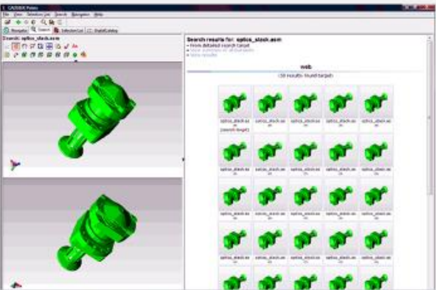
Family members -- or items with topology similarities -- as identified and displayed in CADseek's result-navigation window.
